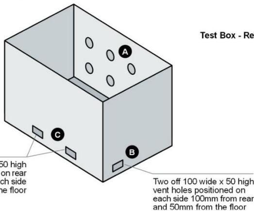
Two off 100 wide x 50 high vent holes positioned on rear face 250mm from each side and 50mm from the floor
